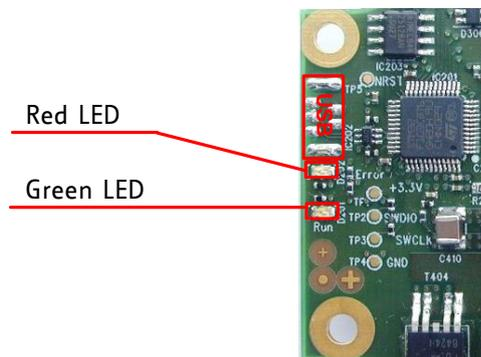
Figure 5.1 on-board LEDs
