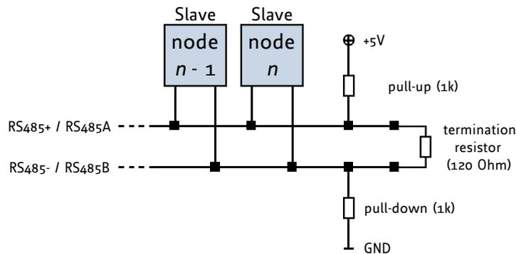
Figure 3.6: RS485 bus lines with resistor network
